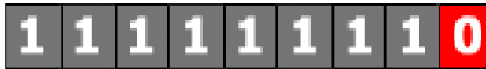
Fig. 11 Supplementing the 9th bit – the indication that the number of transitions was not minimized
